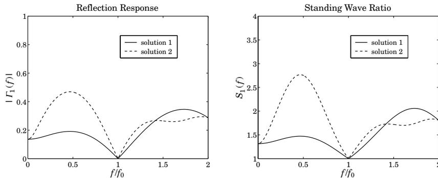
Fig. 11.7.2 Reflection response of two-section series transformer.
