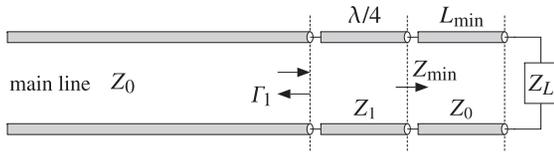
Fig. 11.5.1 Quarter-wavelength transformer for matching a complex load.
