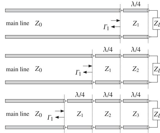
Fig. 11.3.1 One, two, and three-section quarter-wavelength transformers.
