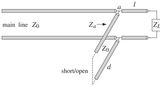
Fig. 11.8.1 Parallel connection of single stub tuner.
