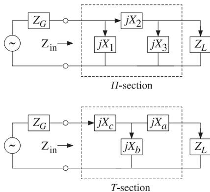
Fig. 11.12.1  $\Pi$ - and  $T$ -section matching networks.
