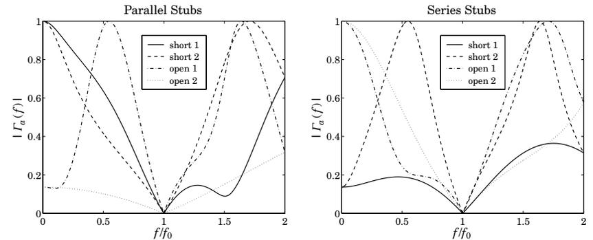
Fig. 11.8.3 Reflection response of single stub matching solutions.
