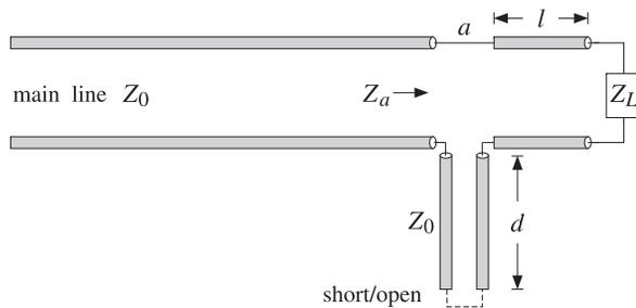
Fig. 11.8.2 Series connection of single stub tuner.
