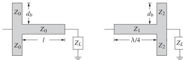
Fig. 11.9.2 Balanced microstrip single-stub and quarter-wavelength transformers.
